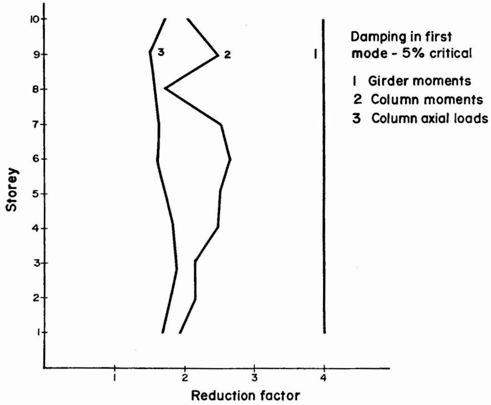
FIG. 10 REDUCTION FACTORS IN TEN STOREY FRAME
