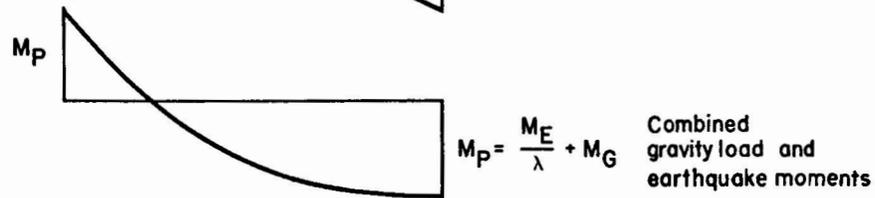
(c) Elasto-Plastic Frame, Gravity and Earthquake Moments
