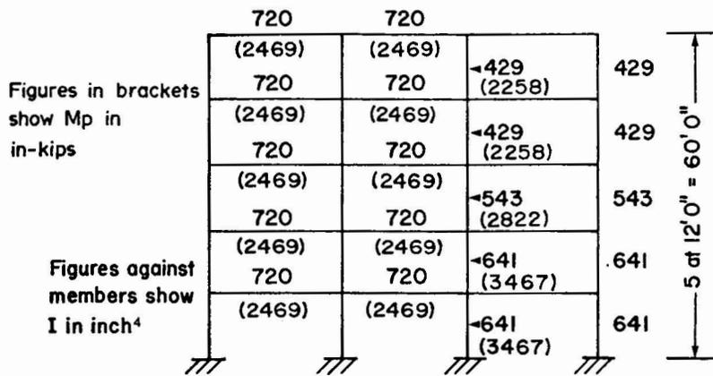
(b) Section A-A and Preliminary Design of Frame I
