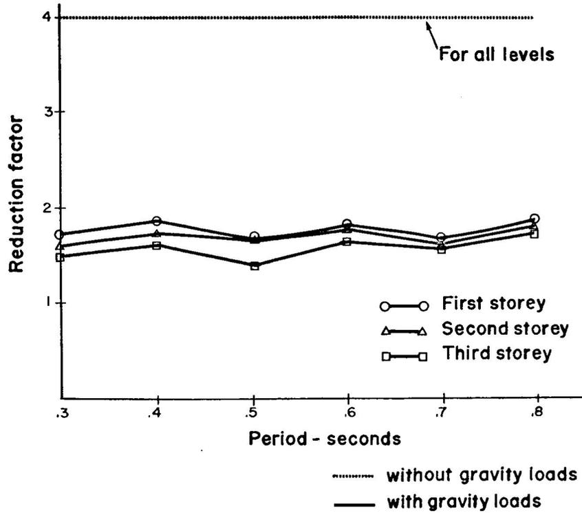
FIG. 6 REDUCTION FACTORS FOR COLUMN AXIAL LOADS IN THREE STOREY FRAME
