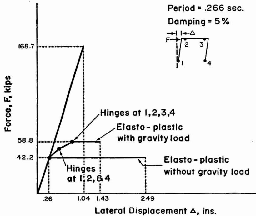
(b) Response of a typical single storey frame
