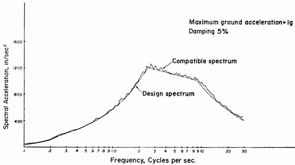
FIG. 1(b) DESIGN SPECTRUM AND ACCELERATION SPECTRUM
